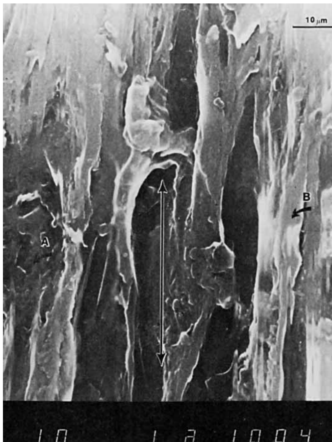
Fig. 3. Electron micrograph showing the non-uniform deformation along the extrusion direction for polystyrene; A, undrawn; B, highly drawn. Long arrow indicates the extrusion direction.
