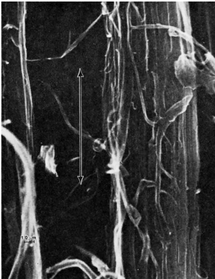
Fig. 2. Electron micrograph showing the fibrous nature of polystyrene oriented by solid-state extrusion. Magnification as indicated. Long arrow shows the extrusion direction.
